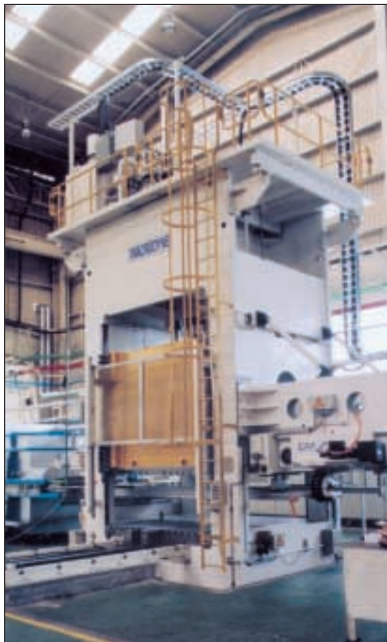
A 1100-ton, four-station hydraulic transfer press line from Macrodyne produces bumpers for an automotive supplier.
