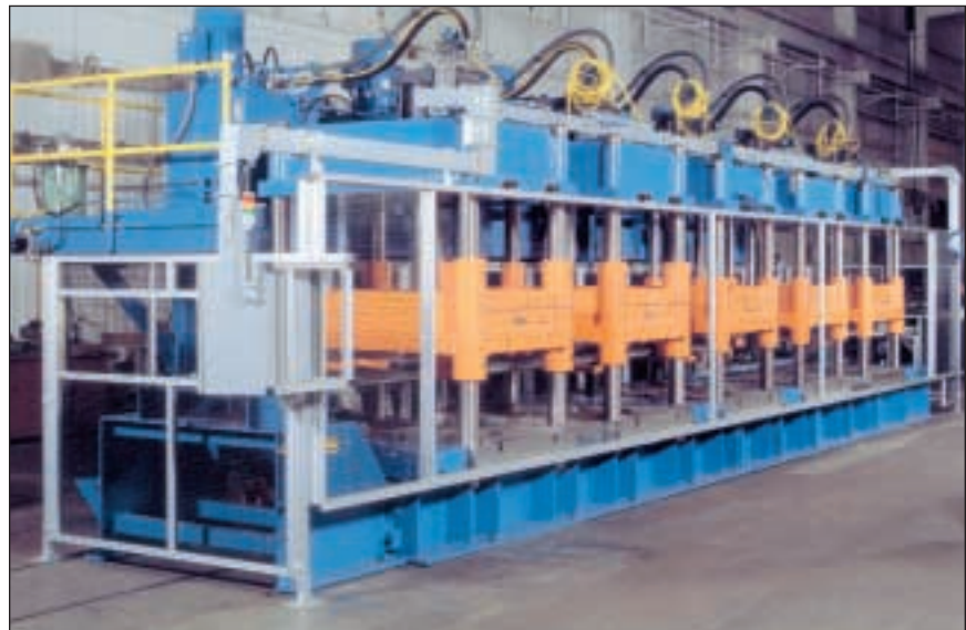
A hydraulic five-press system from Capitol Technologies Inc. helped a manufacturer of steel tool cabinets produce two types of drawers, each with different sizes and depths. The system produces a drawer every 20 sec. while using only two operators.
